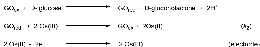
Figure 46. Electron transfer pathway between osmium shuttle and glucose oxidase (GO).
